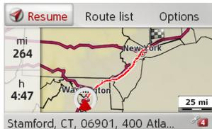
The entire route is displayed. On the left-hand side you can see the distance to be traveled and estimated journey time. The destination address appears at the bottom of the display.
