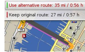
The display provides you with an overview of the alternative route calculated. The red route or route marked purple for an obstruction shows the previous route. The route marked green displays the alternative route calculated. In the upper section of the display, you can see for the previous route and the alternative route the distance to be traveled and the estimated journey time.
