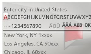
The characters input using the input menu are displayed in the top line of text. The middle section is used for character entry. The bottom section can display a list of all cities corresponding to the letters entered so far when entering a city, for example.
