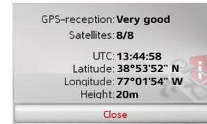
You can see how many satellites are being received, and whether the satellite reception is good enough for navigation. The current time and the geographical position are also displayed.
